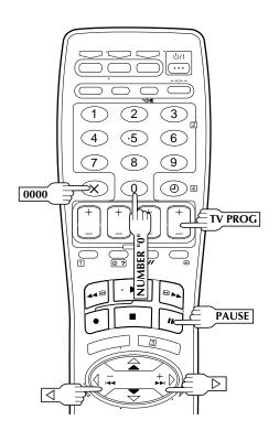
Insert editing replaces part of the recorded scene with new material. Both the picture and Hi-Fi audio soundtrack are replaced with new ones, while the normal audio soundtrack remains unchanged. If you wish to change the normal audio track as well, use the audio dubbing function simultaneously. Use your video recorder as the recorder.
